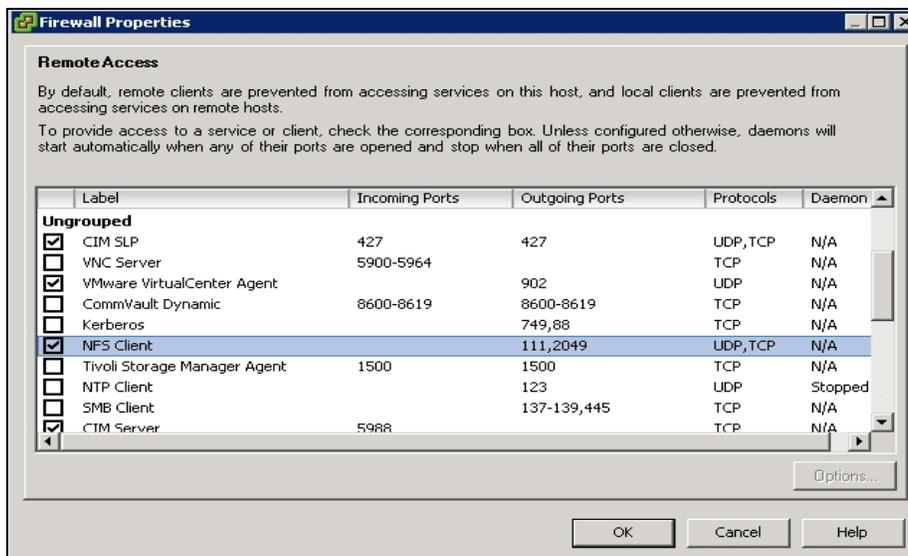
Figure 10.14 - ESX Firewall Properties
