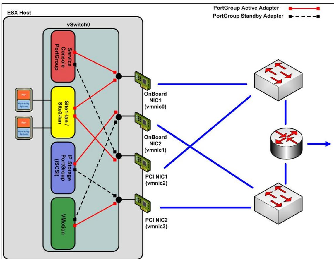
Figure 9.5 – Expanded Core Network Design Example
