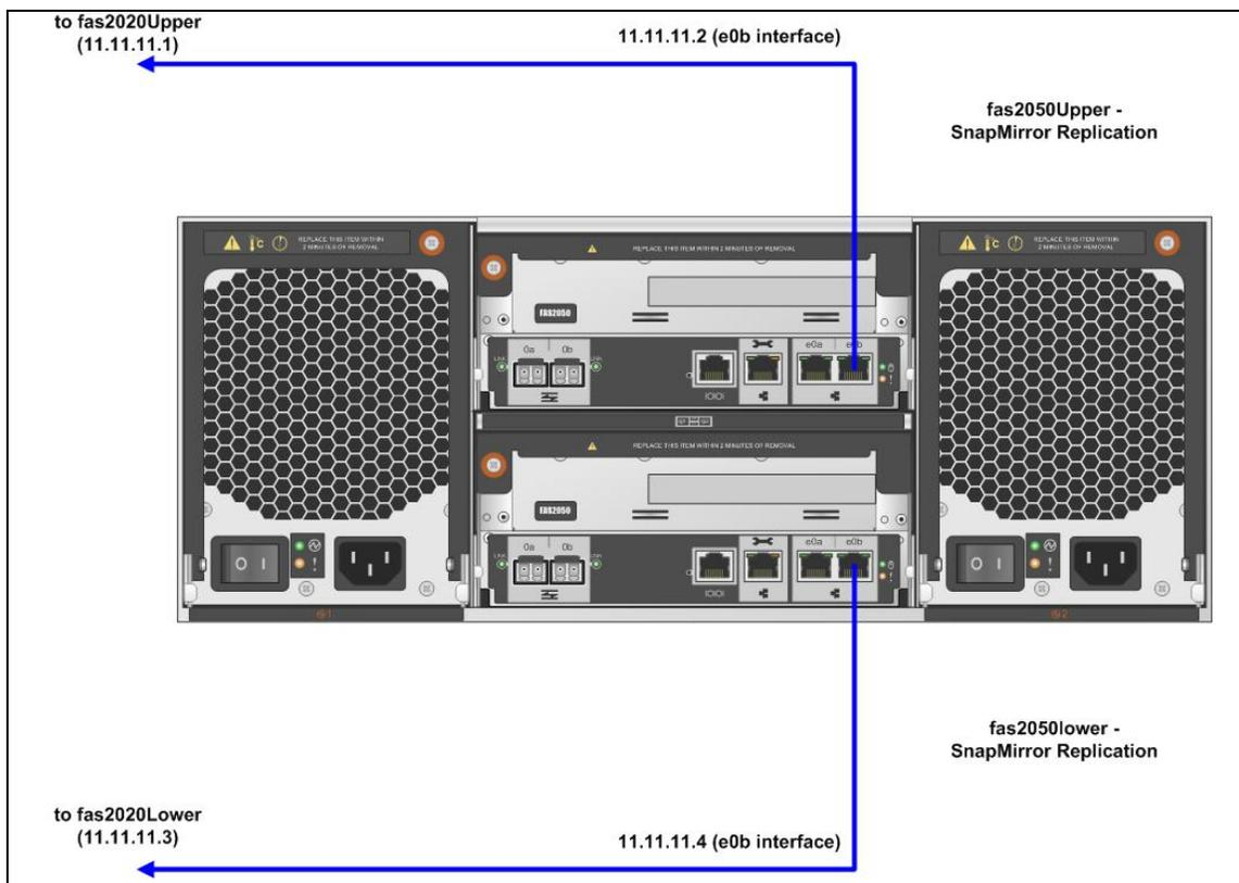
**Figure 10.22 - Site 2 FAS Replication Connectivity**
