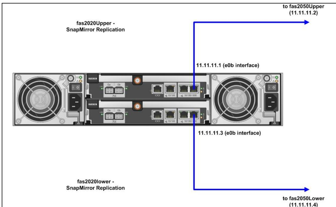
**Figure 10.19 - Site 1 FAS Replication Connectivity**
