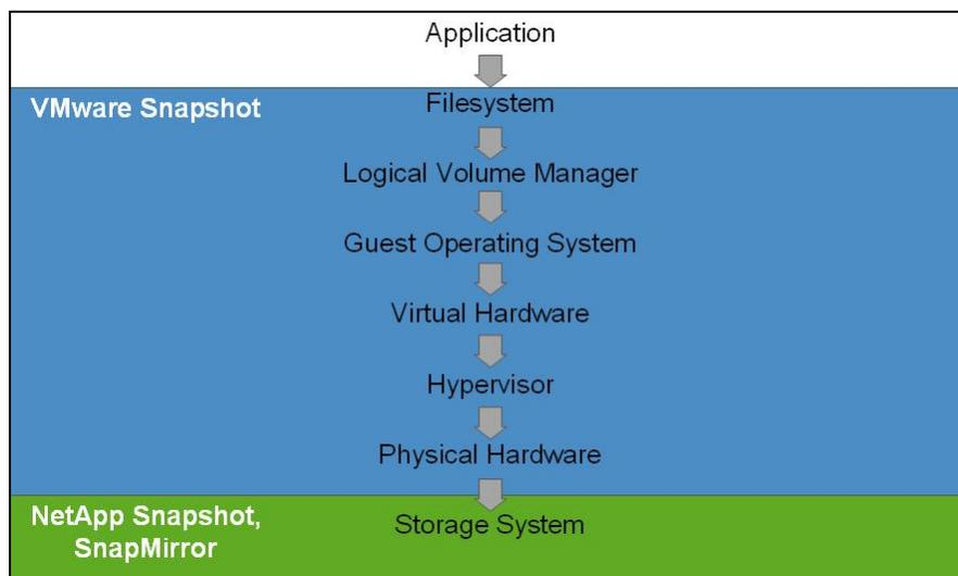
**Figure 11.13 - SnapMirror coordination with VMware snapshots**
