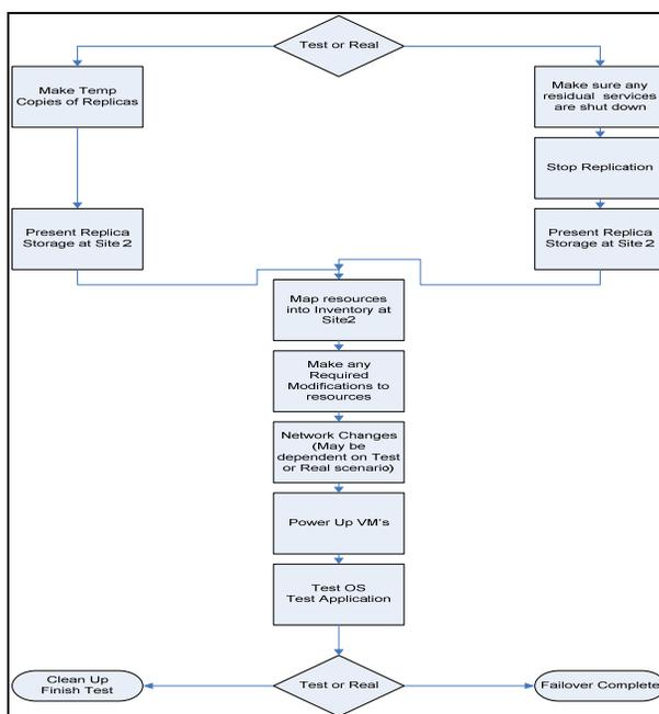
Figure 8.1 Basic Flow of Virtual Infrastructure Recovery/Test
