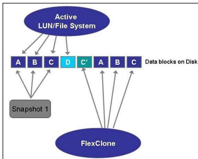
**Figure 11.43 - FlexClone Data Blocks After Split Operation**
