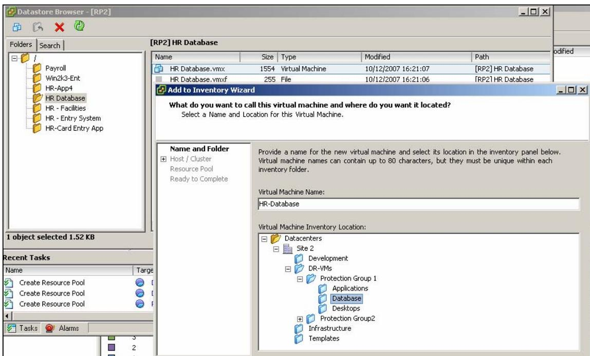
Figure 5.15 - Selecting the Virtual Machine Folder Destination
