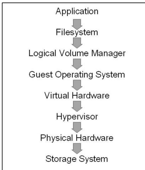
**Figure 11.12 - I/O path in a virtual infrastructure**
