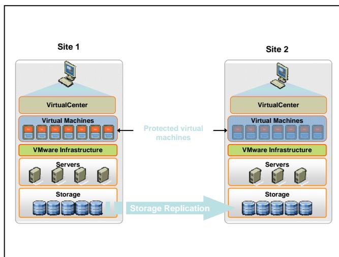
**Figure 5.1 – Virtual Machine Storage Replication**
