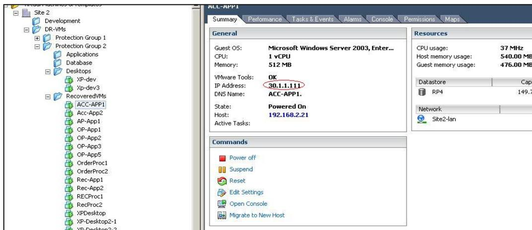
Figure 5.27 - Virtual Machine Network Reconfiguration
