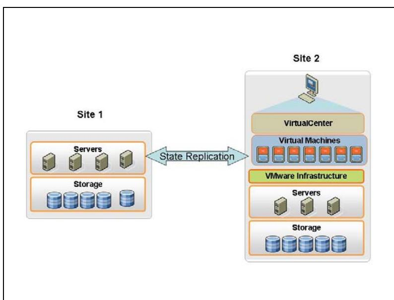
**Figure 6.2 - State Replication with a Single VirtualCenter Instance**
