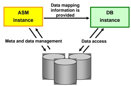
DB instance performs actual access to data files by using the data mapping information from the ASM instance.
