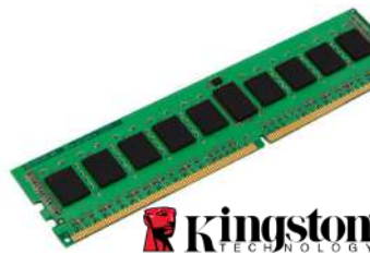
Figure 4 – Kingston's Server Premier - DDR4 - 32 GB - DIMM 288-pin – registered memory module
