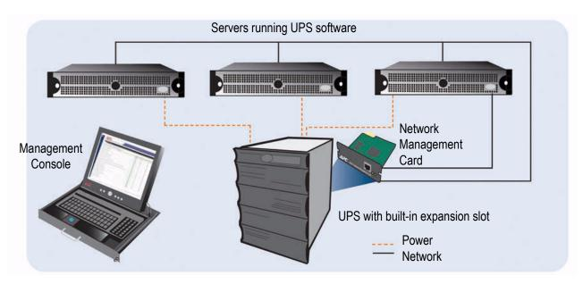
Figure 3 – Protecting three or more computers with a single UPS
