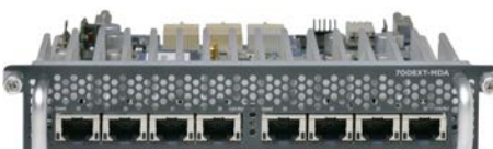
7008XT Media Dependent Adapter featuring 8 x 10GBASE-T ports
