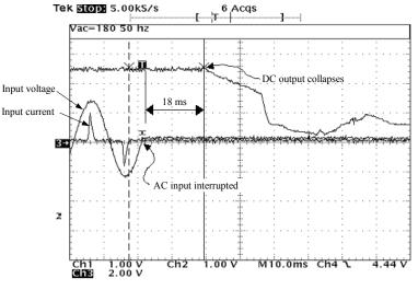
After the AC goes away, a heavily loaded computer power supply's output collapses, but only after a significant delay.
