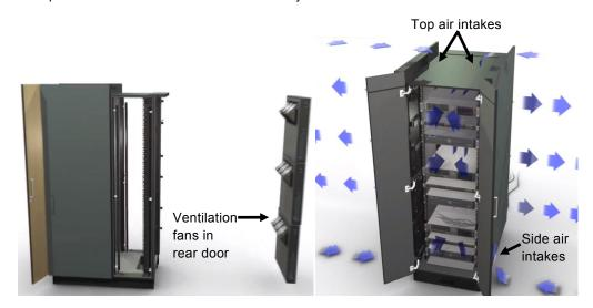
A good practice for reliable cooling is to organize IT equipment in a rack (air intakes are all facing the front of the rack) and use blanking panels to fill in the gaps where there is no equipment. This practice helps prevent thermal shutdown events and reduces the need to overcool the space with oversized air conditioners. Not placing IT equipment in a rack, often allows the hot exhaust air of one chassis to blow into the intake of another.
